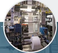
**5.** The resin is drawn down to the proper thickness, air is added forming a bubble which sets the width of the liner.
