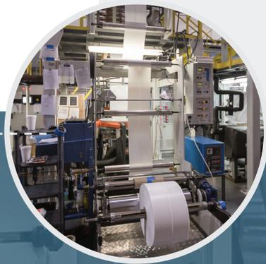
5. The resin is drawn down to the proper thickness, air is added forming a bubble which sets the width of the liner.
